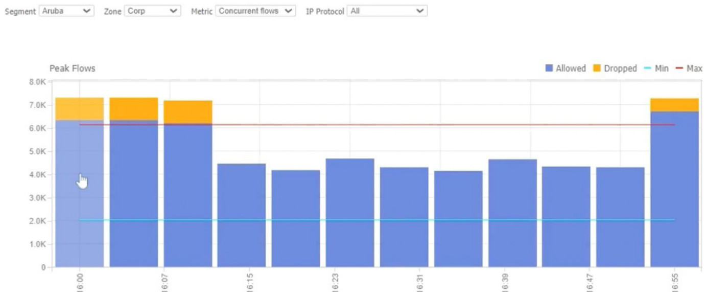
Figure 4. Number of flows allowed and dropped for each 5 minute time interval per firewall zone in HPE Aruba Networking EdgeConnect SD-WAN
